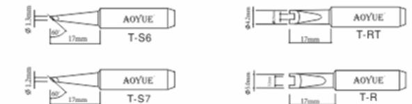
Suitable for all AOYUE soldering irons except lead free composite tip series, induction series and 938
